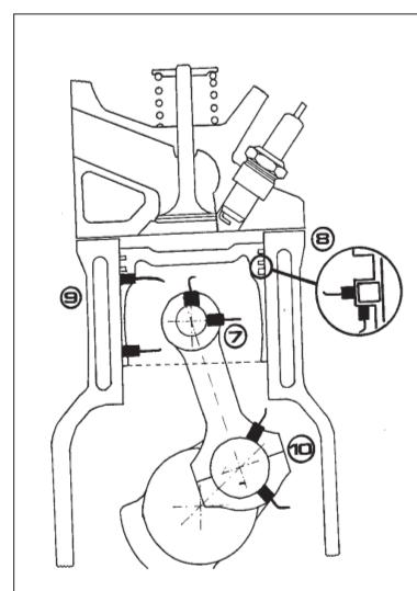
The sensor cable must be laid from the moving piston to the engine block by a special crank arm.
