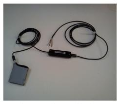
Note the ferrite cores are fitted to the SGIM & AIM unit as a precaution for noisy industrial applications.
