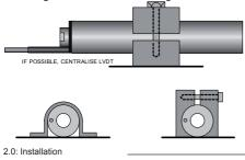
The S-Series transducers contain an integral magnetic screen that reduces these effects. However, the transducer should be positioned well away from electric motors, relays and permanent magnets. If this is not possible checks should be made on the influence of such items.
