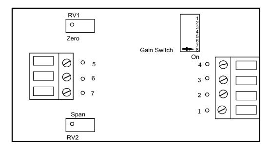
Fig. 3.3 - Gain Selection Switch 8
