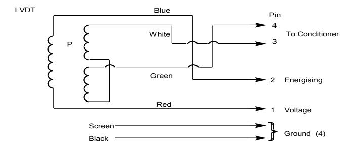
Note: The black lead should only be connected if the transducer case is to be grounded.
