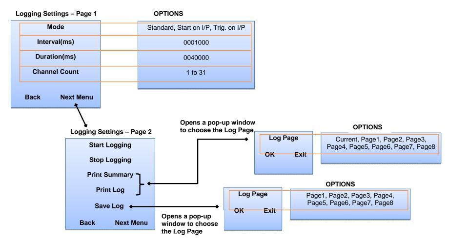
This menu screen allows user to configure the required logging settings. The required number of channels for logging can be selected through "Channel Count" option. NOTE THAT the "Duration" and "Interval" time values have to be multiple of 20ms. User can log up to 8 sets of data onto
