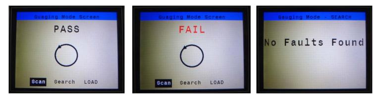
If all the channels selected for scanning are within limits, then "PASS" status is displayed. If one or more number of channels is outside limits, then "FAIL" status is displayed.
