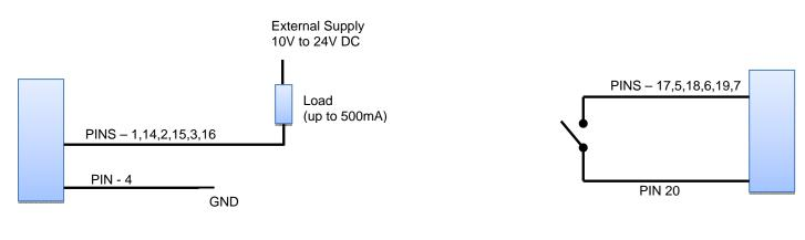
Discrete Outputs Schematic
