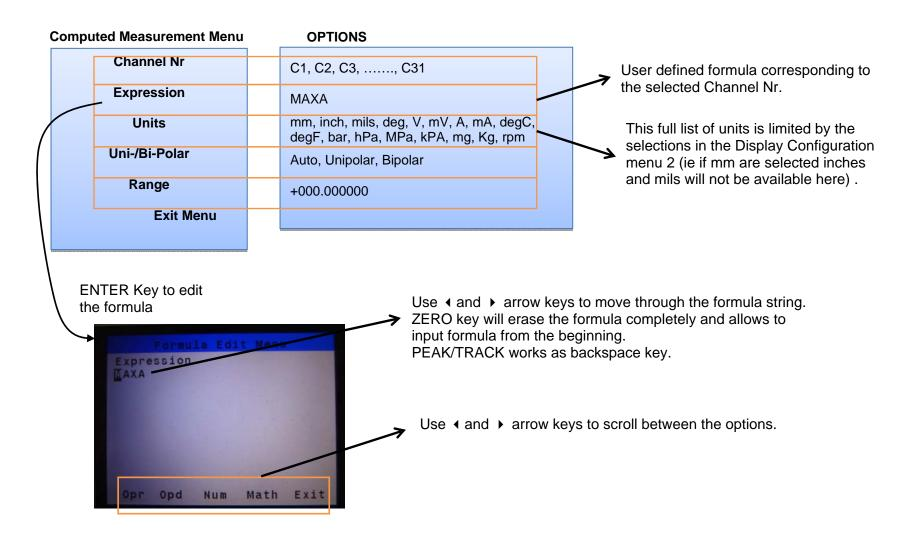
This screen is used to edit/enter the formula for the corresponding channel.
